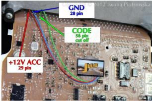
If you want to have engine diagnostics, DO NOT CUT pin 56 from the ECU. Instead, disconnect immobiliser or cut pin 10 of immo box.
