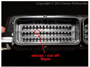
If you want to have engine diagnostics, DO NOT CUT pin 56 from the ECU. Instead, disconnect immobiliser or cut pin 10 of immo box.
