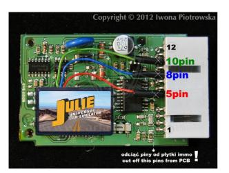
Connect emulator to the socket of disconnected immobiliser:
